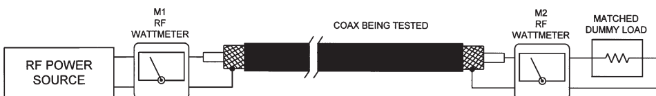
FIGURE 27.22 RF attenuation test setup for coaxial cable.
